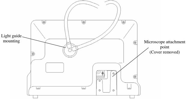
Figure 2 Rear view of the Integraslice
